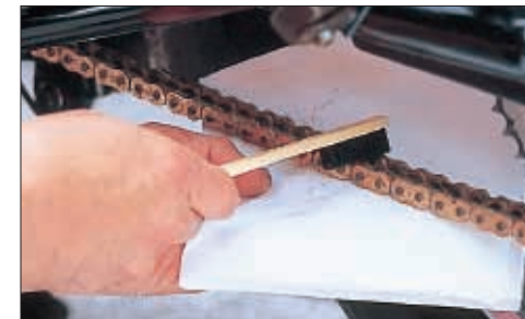
3a. For Non-O-Ring chain ONLY, you may brush away heavy dirt with a soft brush. Even a soft brush might damage O-Rings and X-rings, so please do NOT use a brush on sealed chains. And never use wire brush.
