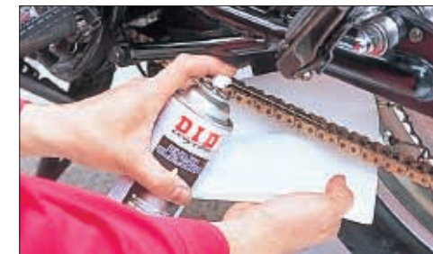
7a. Before spraying on the chain lube, put a tray under the chain and hold a towel behind the chain to prevent overspraying on the motorcycle. Put the motorcycle on stand to allow rotating the rear wheel. When spraying on chain lube, keep the can nozzle a distance of between 2" to 4" away from the chain. While spraying, rotate the rear wheel by hand to coat the entire chain.
