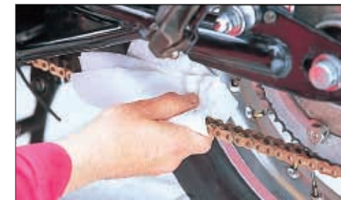
8a. After spraying on the chain lube, wipe the chain with a soft towel to remove excess chain lube. Rotate the rear wheel by hand and wipe the entire chain.
