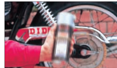
6a. Shake the chain lube can a couple of times to mix up the ingredients.
