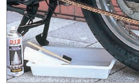
1a. Items needed to clean your chain; chain cleaner, soft towel, tray and for Non-O-Ring chain ONLY a soft brush.
