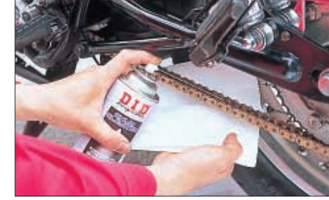
2a. Before applying chain cleaner, put a tray under the chain and hold a towel behind the chain to prevent overspraying. Put the motorcycle on stand to allow rotating the rear wheel. Spray on cleaner while rotating rear wheel by hand to clean the entire chain.
