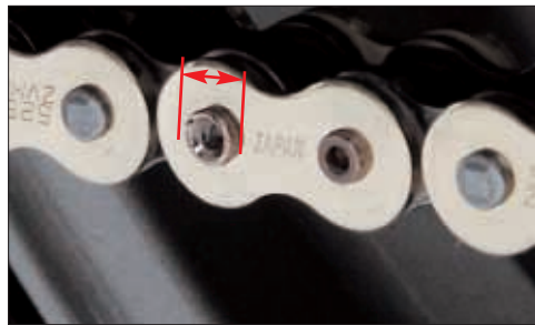
16a. Example of proper flared pin head. If your pin heads are not flared to this extent, Realign chain tool and flare pin heads until they look like the above photo. If your pin heads have cracks or the connecting link is stiff when flexed, remove connecting link and install a new one.
