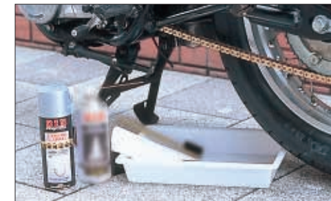
5a. Items needed to lubricate your chain; chain lube, soft towel and a tray.
