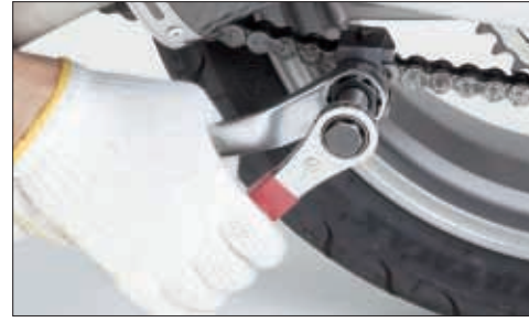
15a. Hold the hexagon part of the tool body with a 27mm closed in wrench, and the bolt head with a 19mm closed end wrench; turn clockwise until the flare part of the pin head makes contact with the surface of the side plate.
