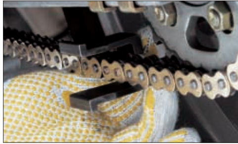
13a. Position the U-shaped holder as seen above. 13b. For clip type (FJ) install the open end of the clip so that it faces in the opposite direction of the chain drive direction.
