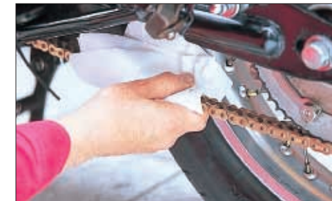
4a. After cleaning the chain, wipe the chain with a soft towel to remove any remaining dirt and chain cleaner. Rotate rear wheel by hand to clean the entire chain.
